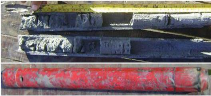
Disturbed sample was taken from SPT tool
